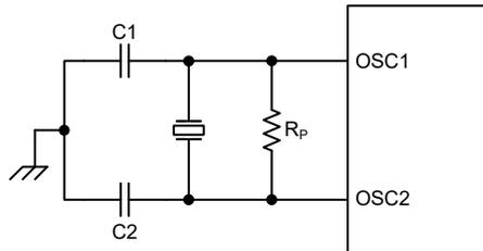
Note: 1.  $R_p$  is normally not required. C1 and C2 are required.
